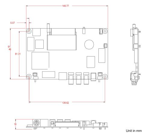
The maximum thickness of the controller is 20.6mm with or without video add-on board (measured from bottom of PCB to top of components, including any underside components & leads). We recommend clearances of:
